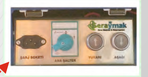
Alt Kontrol Paneli UNDER CONTROL BOX
